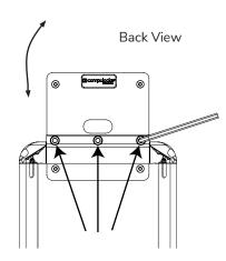
Adjust Tilt Tension by accessing the three screws on the back of the Top End Assembly. Use M5 Hex Wrench (J) to adjust screws.
