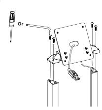
Install Top End Assembly (A) using M5 X 20mm Button Head Torx Screws (B), securing with T-25 Torx Wrench (C).
