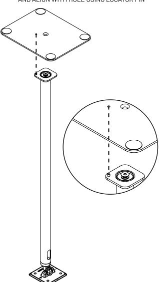
INSTALL THE BOTTOM PLATE USING M10 X 25mm CONICAL ALLEN SCREW (PROVIDED) AND 6mm ALLEN WRENCH (PROVIDED)
