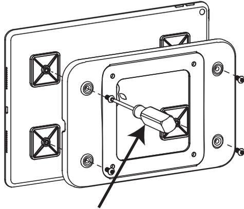
REMOVE MOUNT FROM DEVICE BY REMOVING THE M4 PIN TORX SCREWS USING THE PROVIDED T-15 SCREWDRIVER. THIS EXPOSES THE FOUR (4) ADHESIVE PADS.
