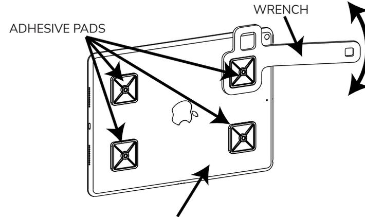
PLACE TABLET OR LAPTOP ON A FLAT PROTECTIVE SURFACE WITH THE 4 ADHESIVE PADS FACING UP. WHILE SECURELY HOLDING THE DEVICE, PLACE THE TOOL ONTO THE ADHESIVE PAD AS SHOWN AND ROTATE WITH STEADY FORCE ALLOWING THE ADHESIVE TO BREAK FREE.
